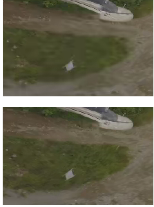
Fig. 3. Ninth frame of the chairlift sequence: visual comparison between HEVC based encoding (top) and geodesic motion model (bottom)
