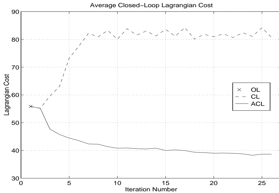
Fig. 9. Performance comparison of standard CL design and the proposed ACL approach to PVQ design. Average Lagrangian cost on the training sequences using the PVQ available at the end of each iteration is shown. Both techniques initially use the outcome of a simple OL design as initialization. Note the gradual decrease in average Lagrangian distortion of the ACL method indicating improvements in the quantizer design. On the other hand, the CL design procedure is unstable.
