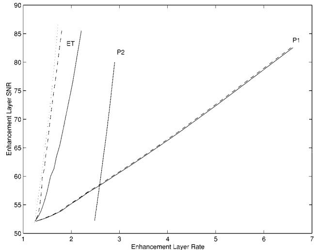
Fig. 7. Performance of two-layer scalable DPCM coding for Laplace–Markov source with  $\rho = 0.95$ . SNR of enhancement-layer versus enhancement-layer rate (bits/sample) is shown for different prediction methods. For P1 and ET prediction, solid lines and dashed lines show performance with single entropy coder and two entropy coders respectively. Base-layer rate was 1.14 bits/sample. Performance of nonscalable coder with the same total rate is indicated by dotted line.
