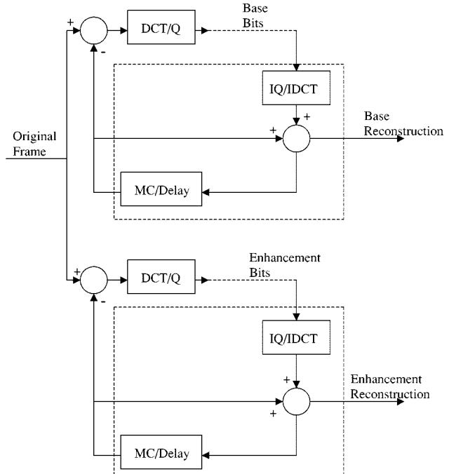
Fig. 3. Sketch of two-layer scalable (en)coder with P2 prediction at the enhancement-layer. Encoder of each layer contains the corresponding decoder (indicated by dotted lines). Transform (DCT/IDCT) and motion compensation (MC) modules are specific to video coding.
