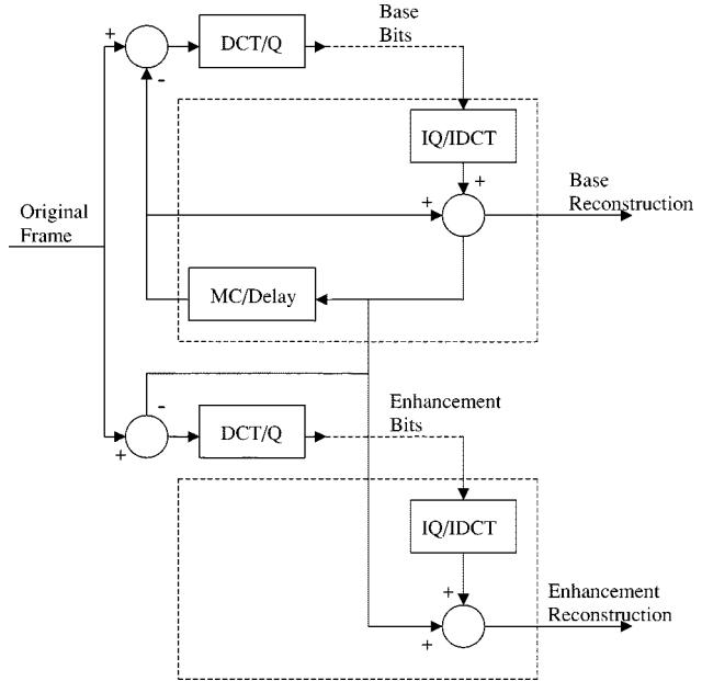
Fig. 2. Sketch of two-layer scalable (en)coder with P1 prediction at the enhancement-layer. Encoder of each layer contains the corresponding decoder (indicated by dotted lines). Transform (DCT/IDCT) and motion compensation (MC) modules are specific to video coding.
