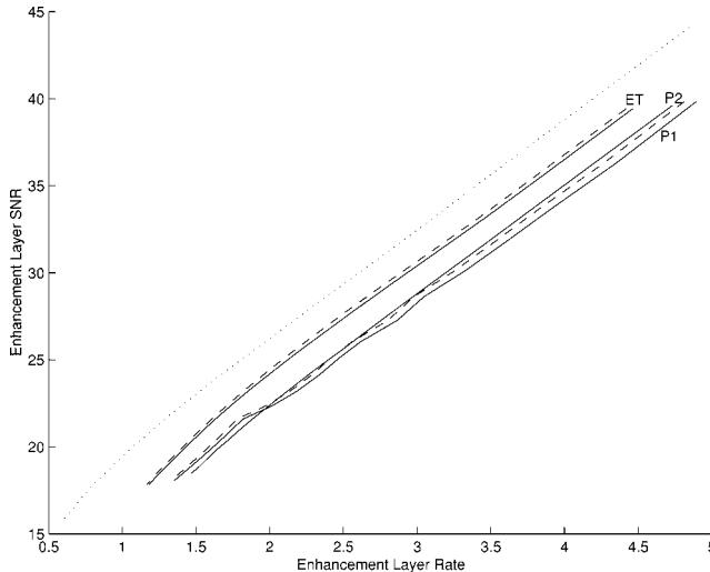
Fig. 6. Performance of two-layer scalable DPCM coding for Gauss–Markov source with  $\rho = 0.99$ . SNR of enhancement-layer versus enhancement-layer rate (bits/sample) is shown for different prediction methods. For P1 and ET prediction, solid lines and dashed lines show performance with single entropy coder and two entropy coders respectively. Base-layer rate was 0.59 bits/sample. Performance of nonscalable coder with the same total rate is indicated by dotted line.
