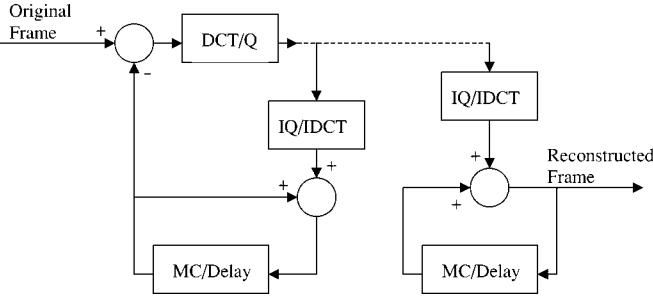
Fig. 1. Sketch of generic predictive coding scheme. Transform (DCT/IDCT) and MC modules are specific to video coding.
