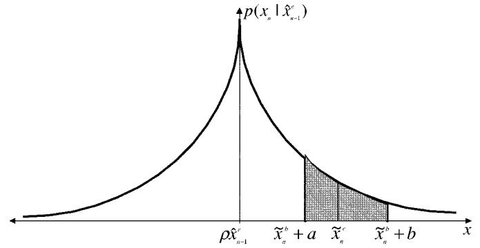
Fig. 4. Computation of ET predictor. The estimate is computed as centroid of the interval specified by the base-layer,  $(a + \bar{x}_n^b, b + \bar{x}_n^b)$ , with respect to the enhancement-layer prediction pdf centered at  $\rho \hat{x}_{n-1}^e$ .
