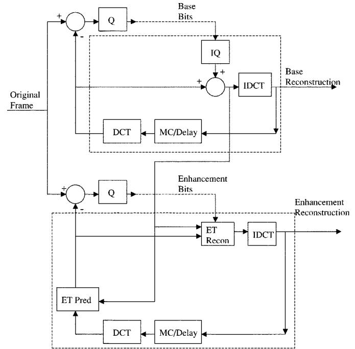
Fig. 5. Sketch of two-layer scalable (en)coder with ET prediction at the enhancement-layer. Encoder of each layer contains the corresponding decoder (indicated by dotted lines). Transform (DCT/IDCT) and motion compensation (MC) modules are specific to video coding.
