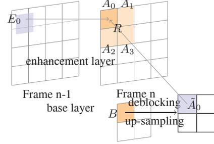
Fig. 1: Pixel domain enhancement layer prediction in spatial SVC.
