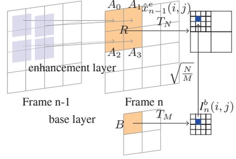
Fig. 2: Estimation-theoretic enhancement layer prediction.
