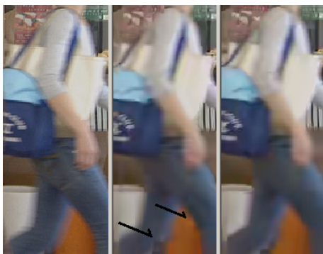
Fig. 4. Visual comparison: a patch from frame 82 in sequence BQMall . (L) Uncompressed; (M) Coded by HEVC reference software; (R) Coded by the proposed methods.
