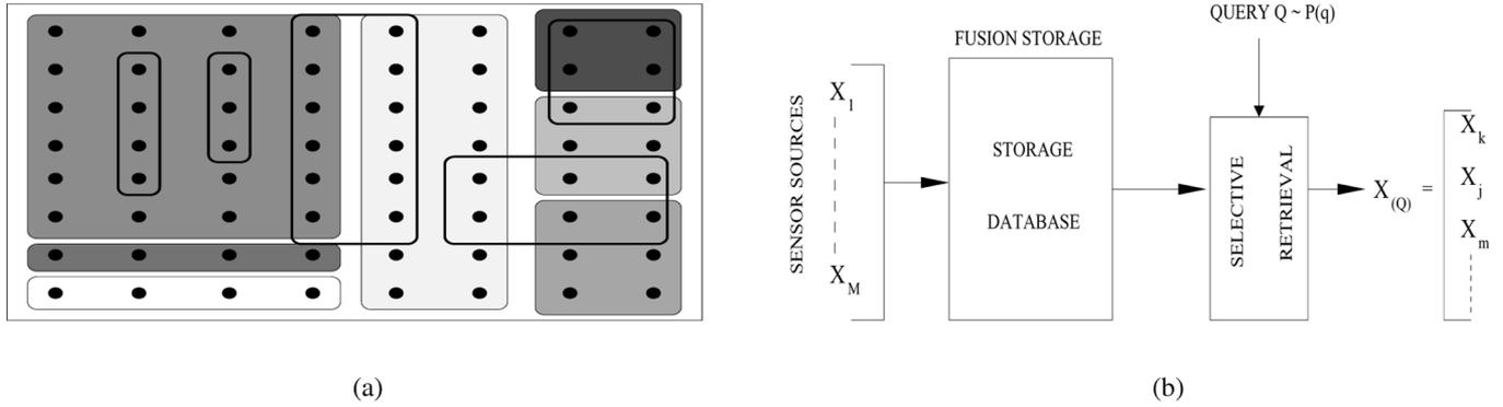
Fig. 1. Fusion coding of correlated sources. (a) A 2D sensor field. Dots represent sensors and boxes represent regions of interest (queries). (b) Fusion storage and selective retrieval.
