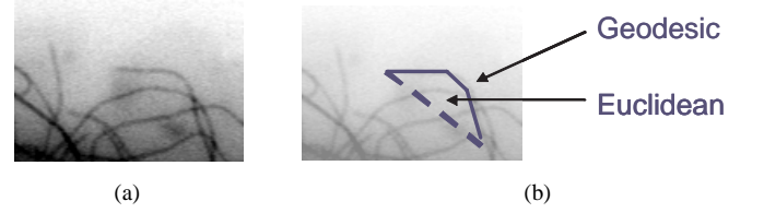
Fig. 2. Estimate of length (a) original, (b) Euclidean vs geodesic.
