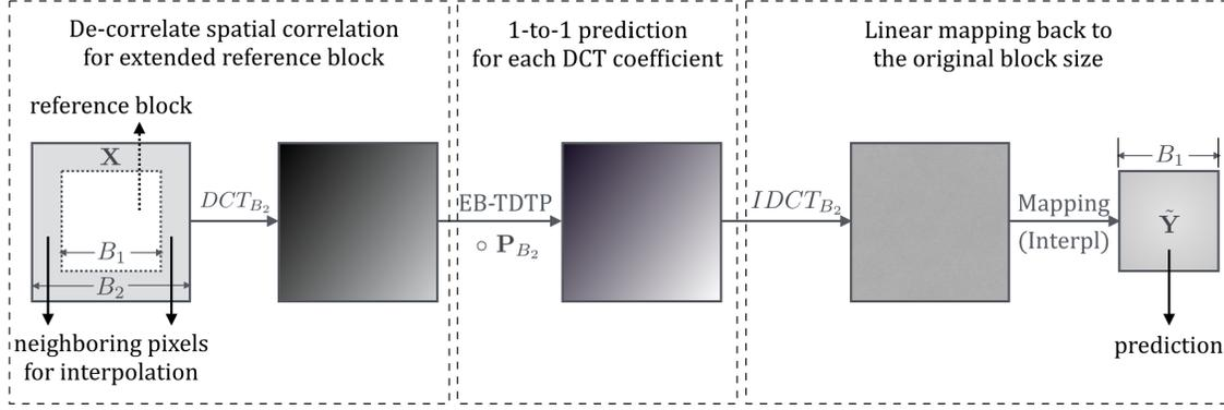
Fig. 1. Block diagram of the EB-TDTP framework
