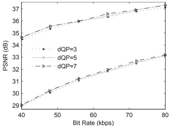
**Fig. 1.** Impact of secondary QP offset, PSNR vs. bit rate (hall monitor, qcif, 10 fps, 40–80 kbps,  $p=10\%$ ). Upper set of curves shows joint redundant encoding and lower set shows general fixed redundant encoding.
