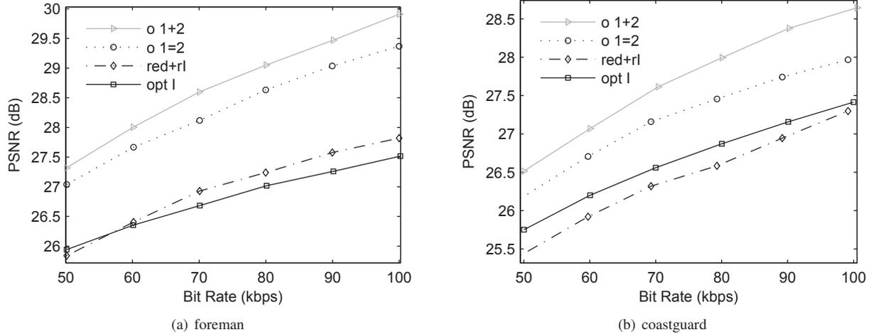
Fig. 2. Delivery performance, PSNR vs. bit rate (qcif, 10 fps, 50-100 kbps,  $p=10\%$ )
