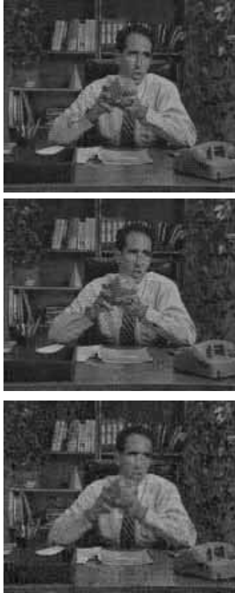
Figure 4. Sample reconstructed frame of “Salesman” for Multimode-JSCC (top), Multimode separate source and channel coding (middle), and Fixed Length-JSCC (bottom) for rate R = 160 Kbps
