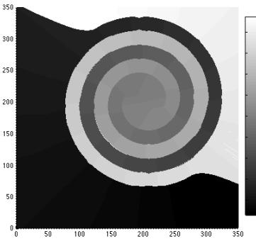
Fig. 4. Obtained mapping for 2:1 Gaussian, CSNR=40dB, SNR=19.41dB. The axes show the two dimensional input ( $\mathbf{x}$ ) and the function value ( $g(\mathbf{x})$ ) is shown as the intensity level.
