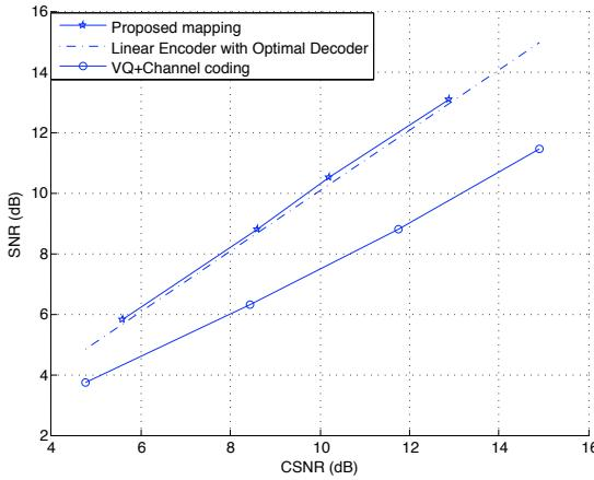
Fig. 7. Comparative results for Laplacian source-Gaussian channel, 2:2 mapping
