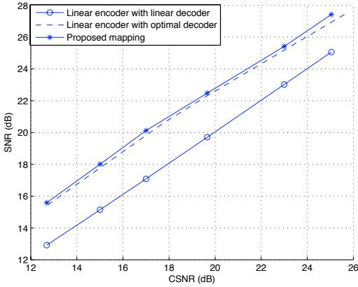
Fig. 3. Comparative results for 1:1 (scalar) mappings, GMM source-Gaussian channel
