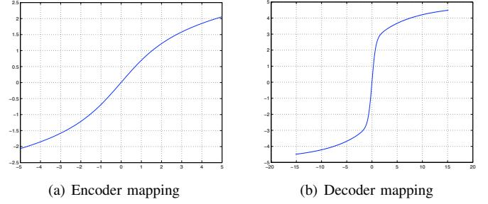
Fig. 2. Example mappings for bi-modal GMM source, Gaussian channel, modes at 3 and -3
