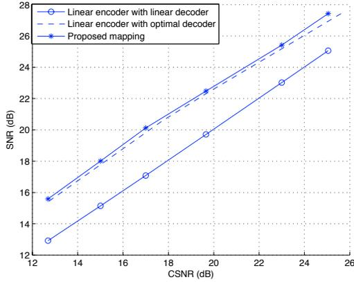
Fig. 3. Comparative results for 1:1 (scalar) mappings, GMM source-Gaussian channel
