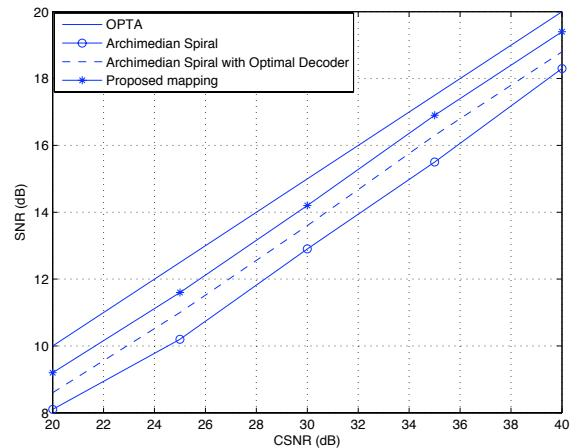
Fig. 5. Comparative results for Gaussian source-channel, 2:1 mapping
