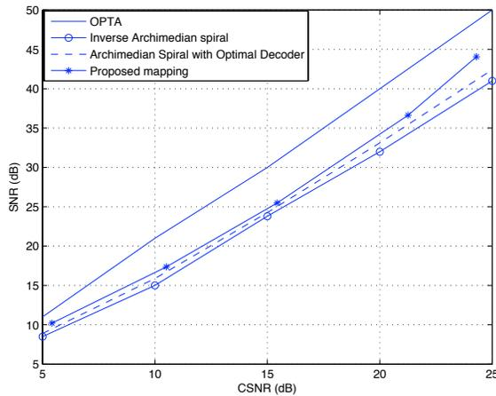
Fig. 6. Comparative results for Gaussian source- channel, 1:2 mapping
