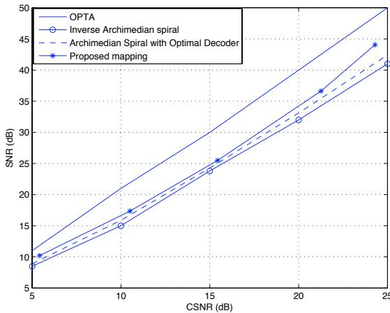
Fig. 6. Comparative results for Gaussian source- channel, 1:2 mapping
