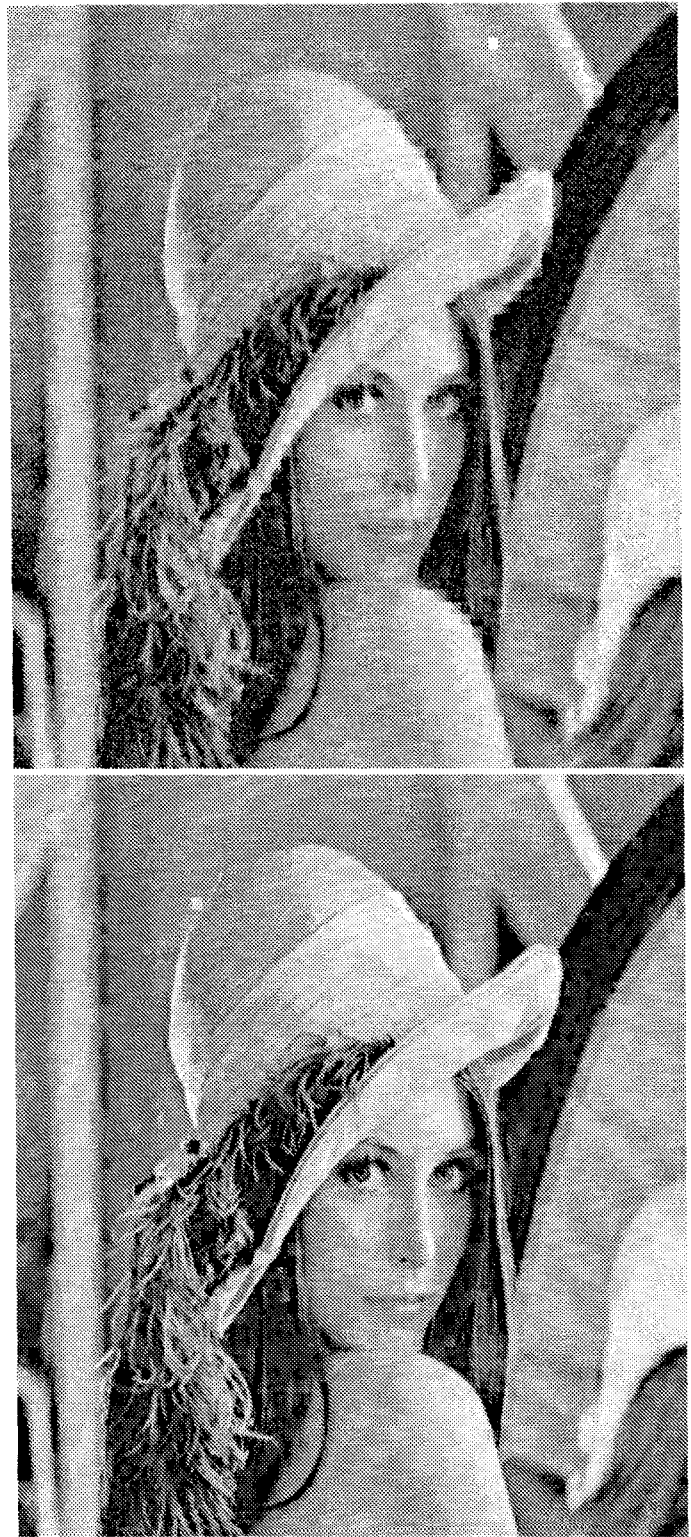
Fig. 1. Performance of MIC-COQ on test image "LENA" for N = 1 (top), and 16 (bottom) modes. The bit rate R = 1.0 bpp and channel error rate \epsilon = 0.005
